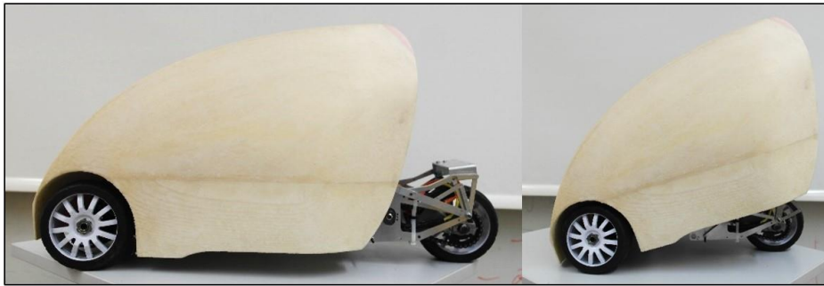
Figure 10: EvoCare Prototype in scale 1:5 including folding mechanism
