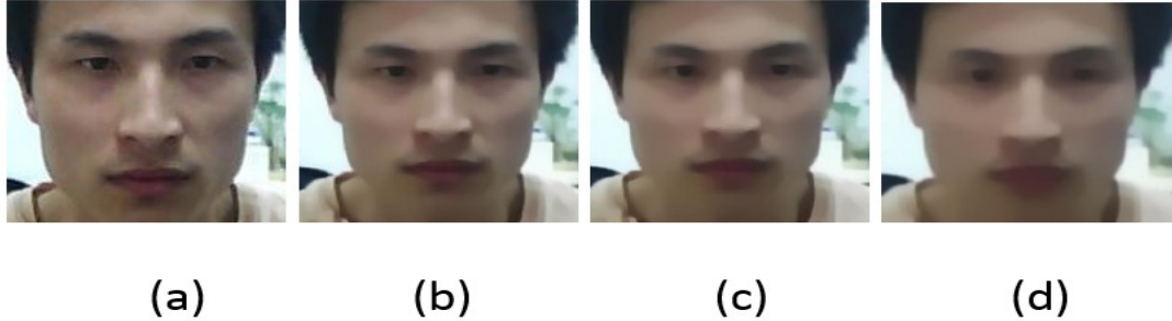
Figure 2.5 Example of diffusion image u^k with different iteration number and time step equals to 10. (a) original image. (b) k = 5 . (c) k = 10 . (d) k = 20 .
