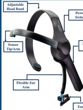
An effective EEG sleep detection technique has been proposed to prove that our algorithm is simple and works fast in real time in an efficient way. The presented approach uses Neurosky Mindwave which is the obtainable, smallest and affordable EEG headset that gathers the user's brain waves.
