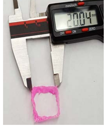
Figure 5. (A) 3D printed square using stained 10% PCL. (B) Final solidified product.[1]
