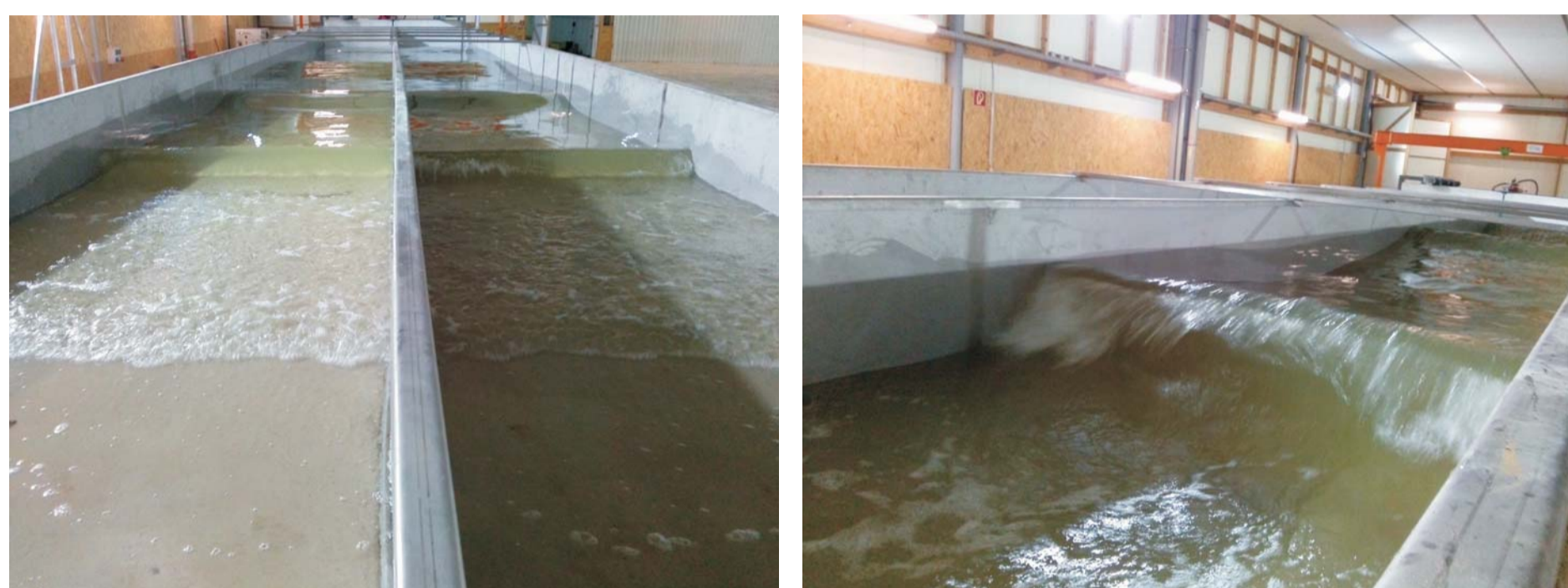
Fig. 1: Wave flume construction as a twin flume with one wave paddle
