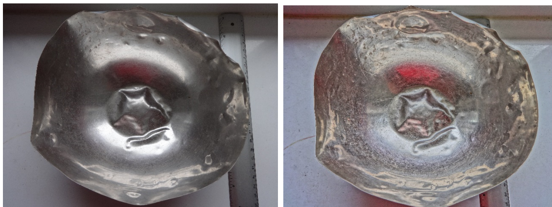
148 149 Fig. 4 A platinum crucible for Auer's heritage. It shows very distinct scratches under right illumination (picture on the right). 150
