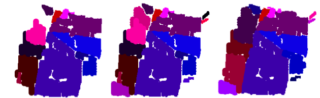
Figure 5. Left: results after adding new segments based on the point cloud to the results in Fig. 4. Centre: results after the second segmentation. Right: results after merging co-planar segments and filling small gaps.
