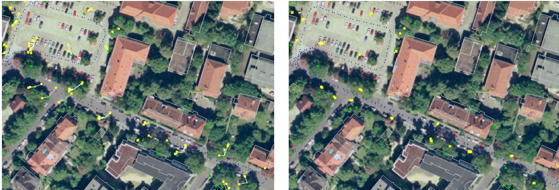
Figure 3: Example snapshots of the interactive association editor. Blue points are the current trajectory, yellow points are poles scanned by ‘Hanna’ (placed using the blue trajectory), green points are the reference poles as extracted from the Streetmapper data, and white lines mark associations between scanned and reference poles. Left: (raw) GPS trajectory with large residuals between associated poles. Right: trajectory based on dead reckoning and pole matching, using the same associations. The residuals were removed largely, leading to a much better trajectory.
