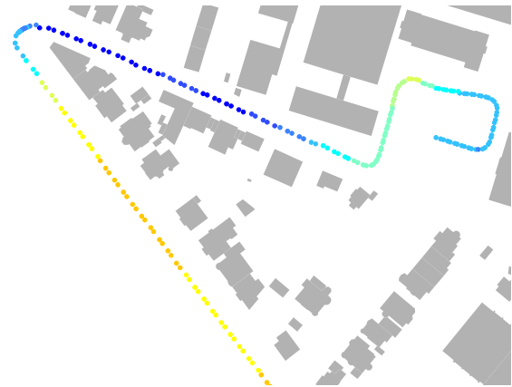
Figure 5: Drift correction applied by the multiple hypothesis filter for a part of run 2. Temperature scale, ranging from -0.34^\circ/\text{m} (red, correction of left drift) to 0.34^\circ/\text{m} (blue, correction of right drift).
