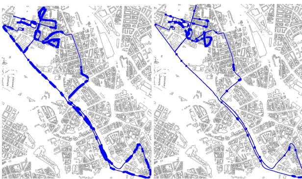
Figure 7: Results of the manual assesment for run 2 (12 km). Bold trajectory points mark erroneous positions. Left: GPS trajectory. Right: Result of matching.
