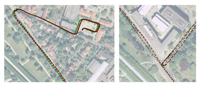
Figure 12: Comparison of original vehicle trajectories (red dots), as obtained from the RTS Hanna GPS/odometry positioning system and corrected trajectories (green squares), using pole matching.
