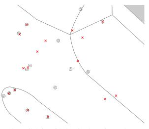
Figure 10: Detailed view of the junction: large distances between extracted poles (red crosses) and ground truth (black circles, radius: inner circle 25 cm, outer circle 50 cm) are not measurement errors but due to a rebuilt of the junction.
