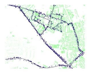
Figure 3: Extracted poles (blue dots) in a larger area with buildings from the cadastral map (green). The thin dotted line is the trajectory of the Streetmapper van.
