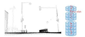
Figure 2: Left: Part of the Streetmapper scene containing a sign post, street (and traffic) light, and traffic light. Right: Illustration of the pole extraction algorithm using a stack of hollow cylinders.
