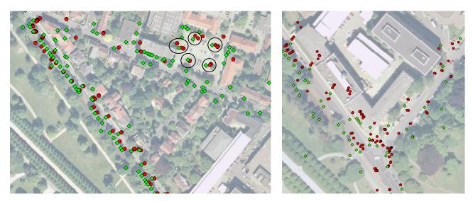
Figure 7: Comparison of reference poles (green squares) and poles extracted using the RTS Hanna vehicle (red dots).
