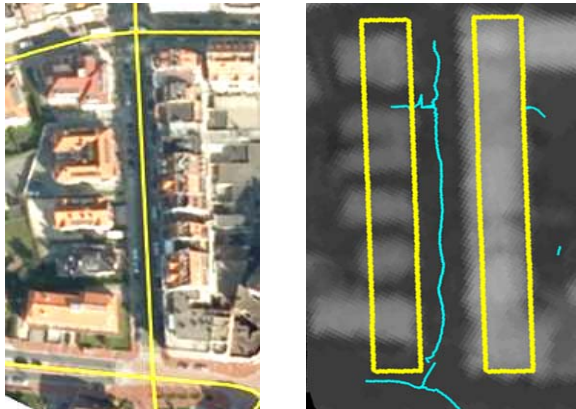
Figure 2: Left: RGB image with database roads. Right: nDSM with 3D-line extraction result (cyan) and region mask for computing entropy (yellow)
