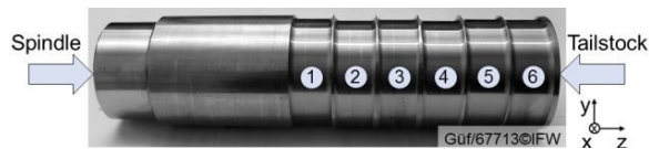
Fig. 9. Shaft for grinding tests with the active tailstock
