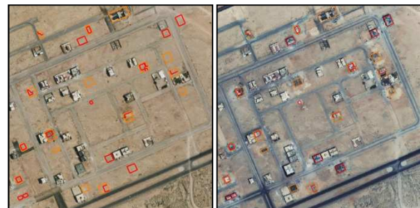
Figure 9. Updated map overlaid with aerial orthophoto from 2007 (left) and IKONOS orthophoto of 2008 used for mapping (right)
