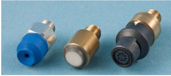
Fig. 4: Vacuum grippers: commercial HT1 suction gripper, special purpose porous gripper (developed at IWF), commercial electronic assembly gripper (left to right)
