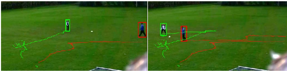
Figure 10. Situation in which a person leaves the field of view for about 8 s. The algorithm manages to keep the correct assignment (sequence from top left to bottom right).
