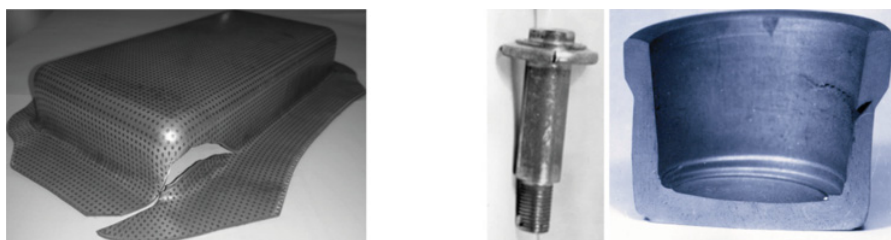
Figure 1. Examples of fracture in sheet (left) and bulk (right) metal formed part.
