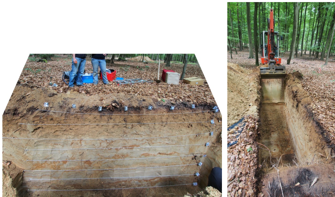
Fig. 1. Image of Transect 2 (left). Lines show the horizontal position of sampling locations A to H ( \Delta x = 45 cm); depth increments \Delta z = 10, 35, 60, 85, 110, 135, 160, 185 cm. The image on the right shows the view directly from the adjacent tree.
