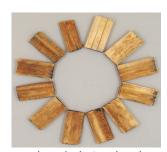
The heartwood samples having a large between-tree variation in the extractive concentrations, and subsequently in the mass loss in a 7-week decay test (the range of mass loss I - 49 %, Coniophora puteana).
