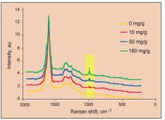
Stilbene content of wood samples was quantified based on the intensity of the band at ca. 996 cm (A.-S. Jääskeläinen/VTT).
