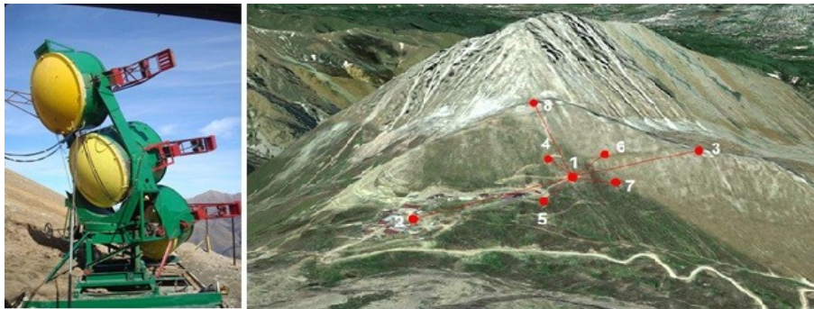
Figure 1: Horizon-T detector: Cerenkov light detectors (left) and charged particles detection points location (right)
