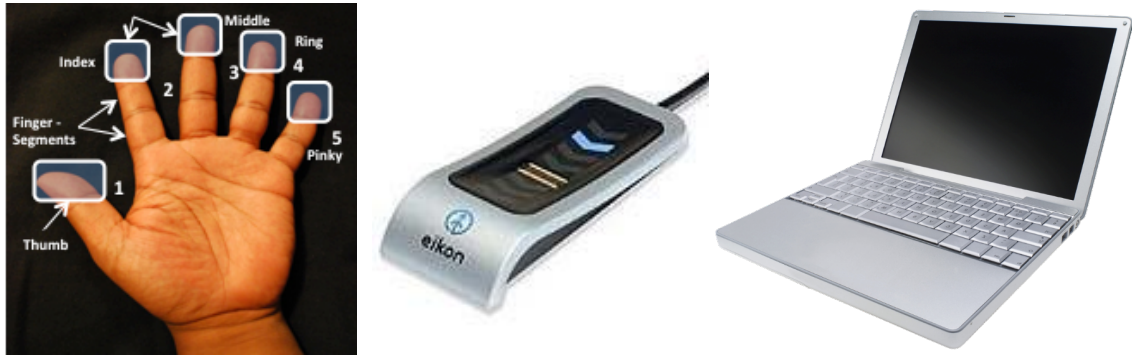
Figure 1. BIO-PIN Authentication System (BIO-PIN Sequence, Fingerprint Reader and Laptop Computer
