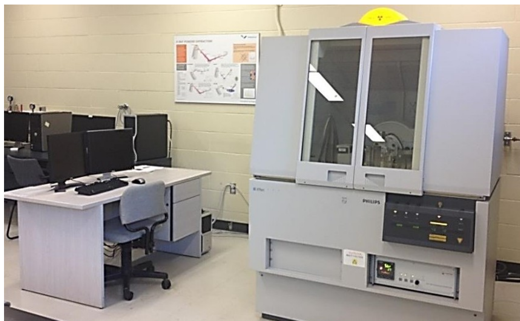
Figure 3.5 The Philips X'pert PRO Diffractometer used for XRD analysis
