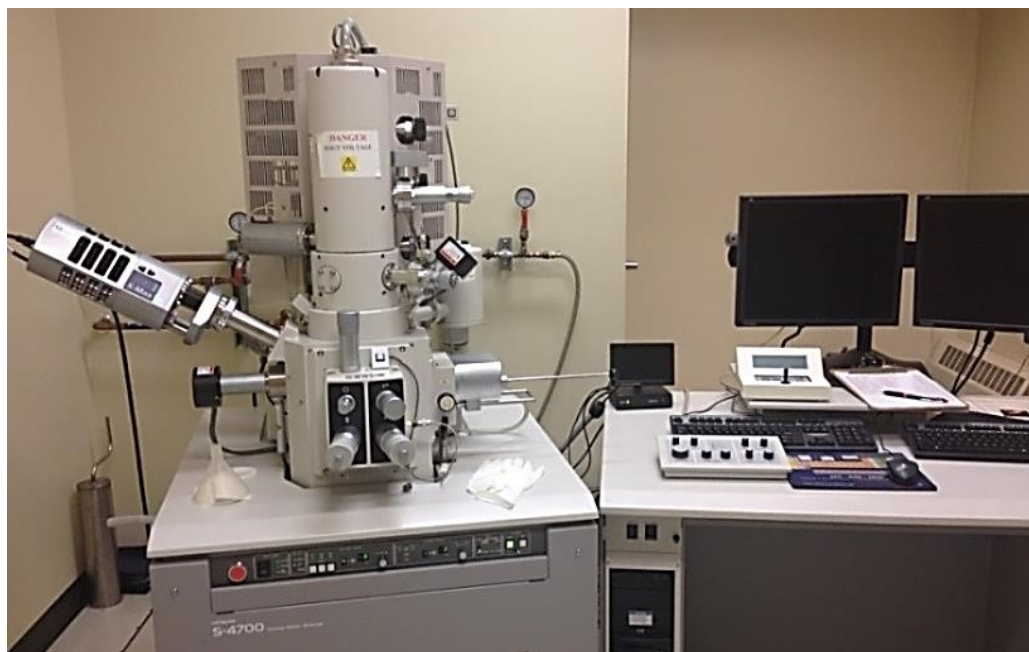
Figure 3.4 The Hitachi S-4700 Scanning Electron Microscope
