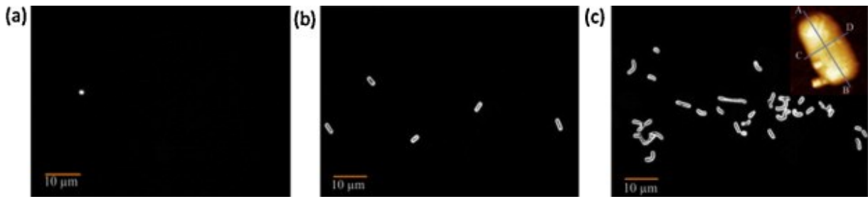
Figure 25. Optical images of the GaAs samples biofunctionalized with E. coli Ab and exposed for 30 min to (a) PBS (1 \times ) solution, (b) 10^5 CFU/mL of B. subtilis (0.1 bacteria/100 \mu\text{m}^2 ), and (c) 10^5 CFU/mL of E. coli (1.1 bacteria/100 \mu\text{m}^2 ). Inset shows an AFM image of an individual E. coli (AB = 2 \mu\text{m} , CD = 1 \mu\text{m} ).
