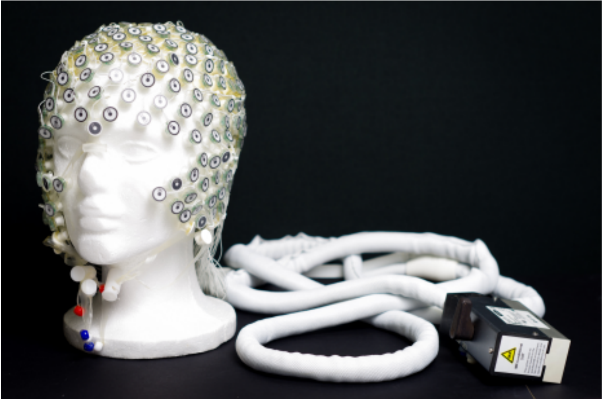
Fig. 1.: An EEG cap shown on a mannequin head. All wires connect to a central unit via the large white cable [46].
