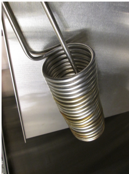
Figure 4.3: Photo of the heating coil manufactured in-house.
