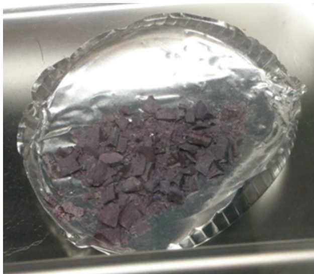
Figure 6.4: Picture of the crushed \text{UCl}_3\text{-LiCl-KCl} salt prior to being loaded into the nebulizer.
