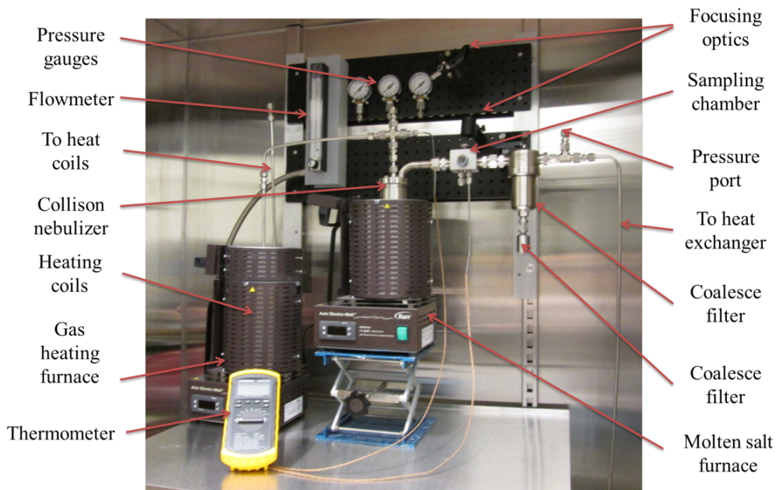
Figure 4.8: Photo of the aerosol system assembly.
