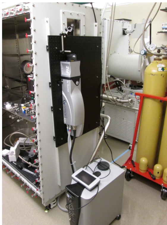
Figure 4.10: Photo of the Q-smart laser mounted to the glovebox and optics used to direct the beam through the window and into the glovebox.
