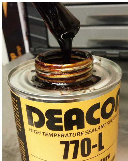
Figure 5.1: Deacon 770-L thread sealant used to seal the NPT threads used to attach the tubing to the sampling chamber.
