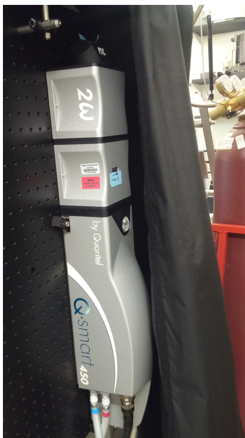
Figure 3.1: Picture of the Q-smart 450 Nd:YAG laser used in this work.
