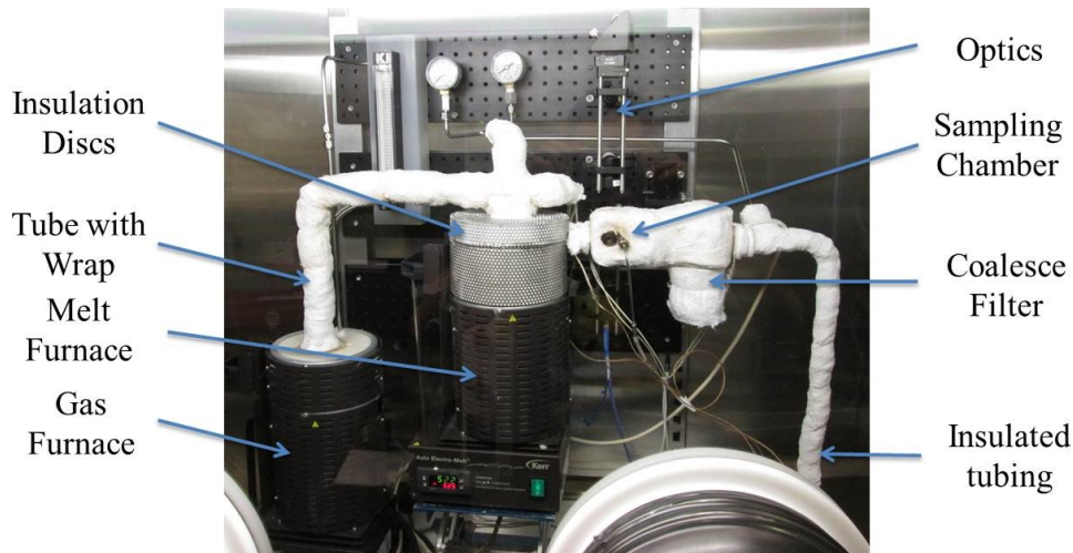
Figure 5.2: Initial high temperature aerosol-LIBS configuration with insulation and heating. prior to operating the aerosol-LIBS system with molten salt.
