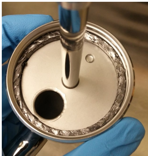
Figure 5.5: Photo showing the inside of the nebulizer lid with the graphite cord placement.
