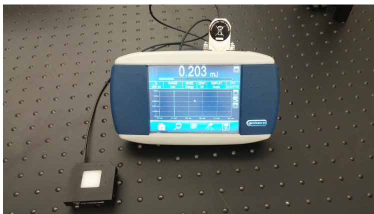
Figure 3.2: Picture of the laser power meter used to determine the laser energy.
