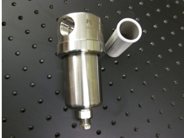
Figure 4.6: Photo of the coalescing filter housing and filter element.
