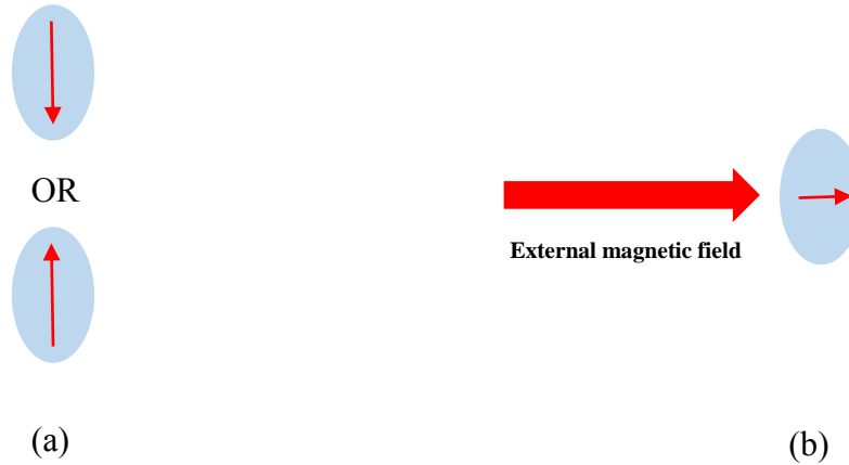
Fig 1.4: Elliptical nanomagnets. (a) The magnetization shown in red tends to align along the major axis, which is energetically favorable.(b) Only on application of external magnetic field along the minor axis, the magnetization is forced to align along the minor axis.
