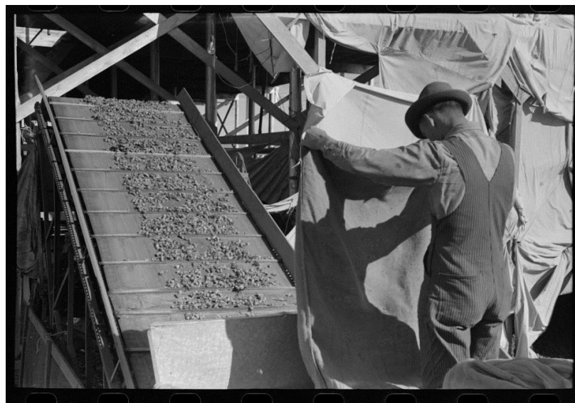
Figure 142. Hops coming from portable-type mechanical picker, Yakima Chief Hop Ranch, Yakima County, Washington. Man empties bags of green hops picked by portable Hop-picker onto conveyor to go through re-picker. (Russell Lee, 1941)
