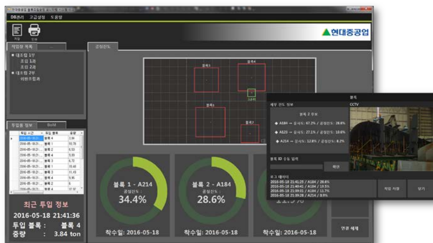
Figure 3.8: The ship block assembly monitoring system
