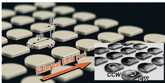
Figure 1 Magnetic imaging of asymmetrically shaped disks. Schematic diagram of asymmetric disks with radius R=500 nm, height h=100 nm and edge ratio r=0.2R within an array with an interdisk distance of d=200 nm. Insets show representations of MTXM images of the in-plane magnetic components observed in a positive field sequence from +100 to 0 mT.
