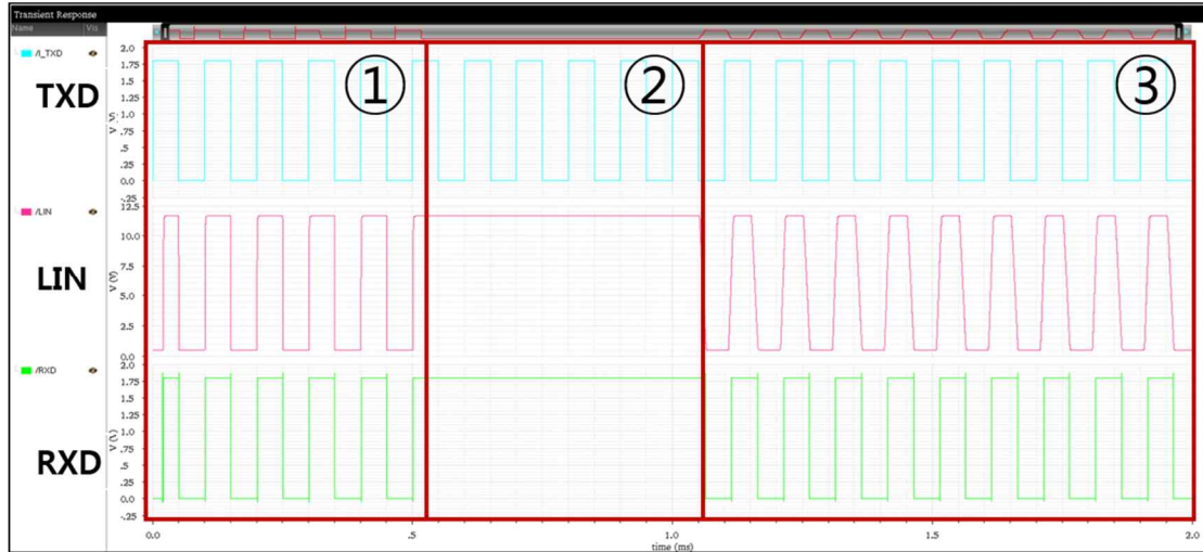
Figure 3-11: Cadence simulation waveform of mode change
