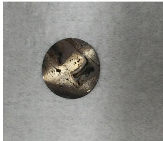
Figure 3-24. The real picture of Ni nanowire current collector made by homemade electrodeposition kit.
