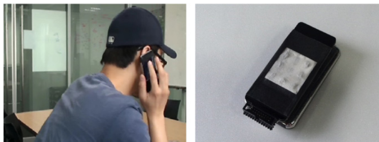
Figure 2 Left: Holding CheekTouch and providing stimulations, Right: CheekTouch device (3x3 vibrotactile motors on the cheek-side, touch screen on the holding finger-side)
