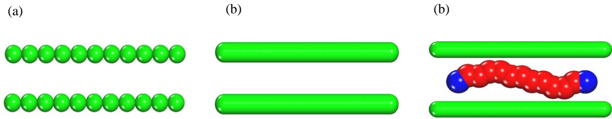
Figure 2.2.2 (a) Realistic wall where wall atoms are successively connected to each other at a specified distance. (b) Ideal smooth wall where wall atoms are connected to each other at an infinitely short distance. (c) Polymer chains are confined in-between the top and the bottom ideal smooth walls.
