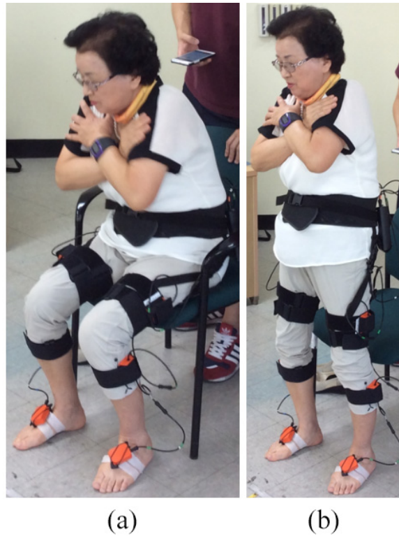
FIGURE 2.6: Experimental setting of sit-to-stand five times test. (a) sitting posture; (b) standing posture.
