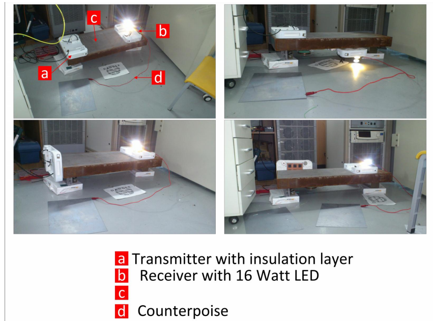
FIGURE 4.9: Power transfer demo: free position.
