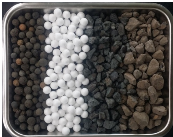
Figure 2. Shape of lightweight aggregates (B700, EPS, ST700, and AS700 from left to right).
