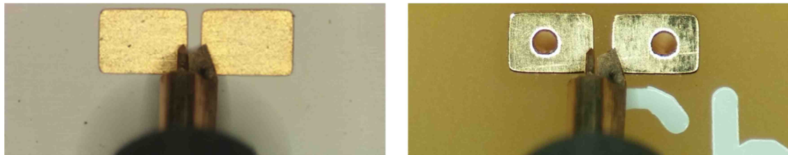
Fig. 2-8. Probing examples: the indirect-contact probing on the dielectric contactor mounted on the DUT or the calibration vias (left) and the contact probing (right)
