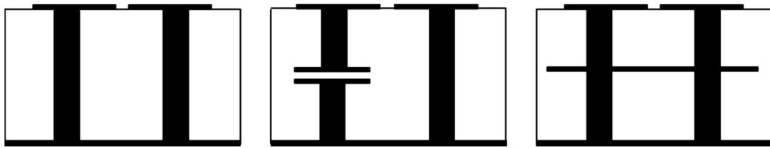
Fig. 2-4. DUTs of (a) the normal via, (b) the open via defect, and (c) the short via defect
