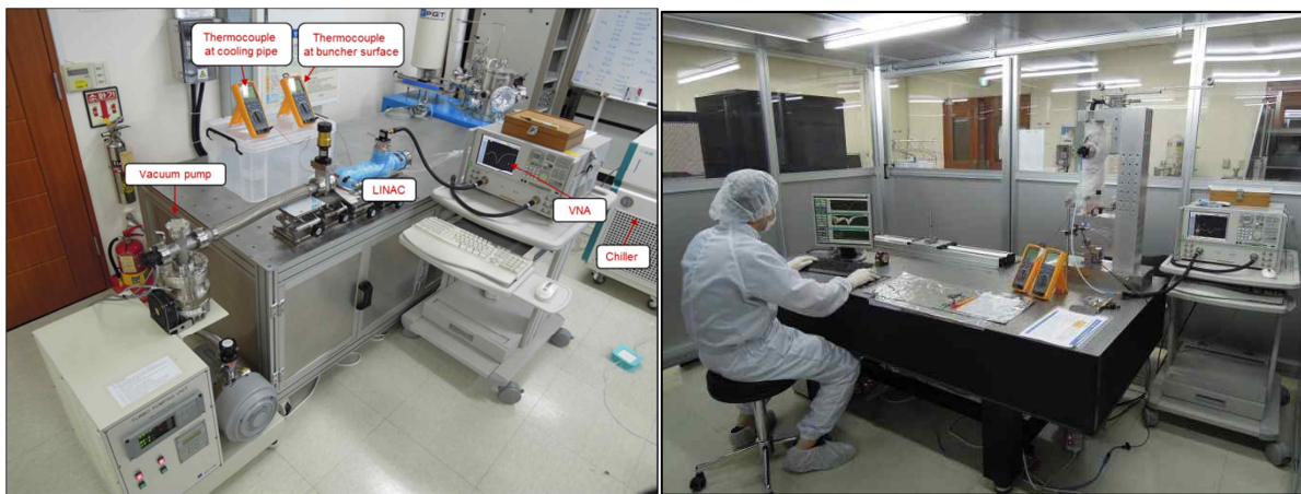
Figure 3.26: Experiment setting for measuring S-parameter and electric field distribution by bead pull of X-band 6 MeV LINAC waveguide
