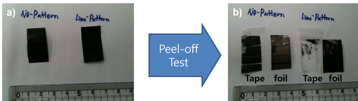
Figure 4. 4 The peel-off test of the patterned and non-patterned \text{LiFePO}_4 electrodes. As expected, the \text{LiFePO}_4 electrodes on the patterned current collectors were strongly attached to the current collectors, while electrode materials were easily peeled off from non-patterned current collectors.
