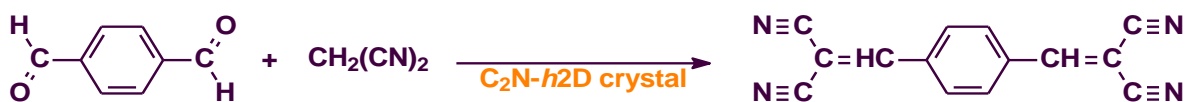
Figure 2.20. Schematic presentation of Knoevenagel condensation reaction of terephthalaldehyde and malononitrile in the presence of the C_2N-h_2D crystal as a reaction catalyst.
