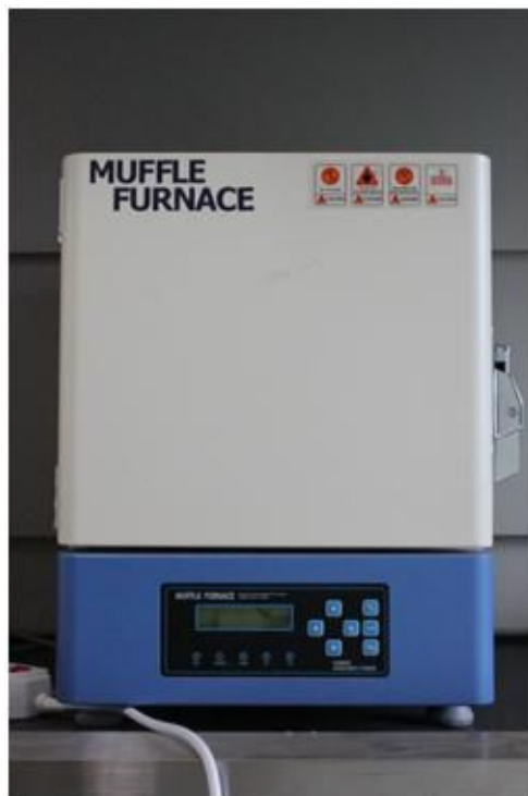
Fig. 4.1 Photograph of air furnace for corrosion test
