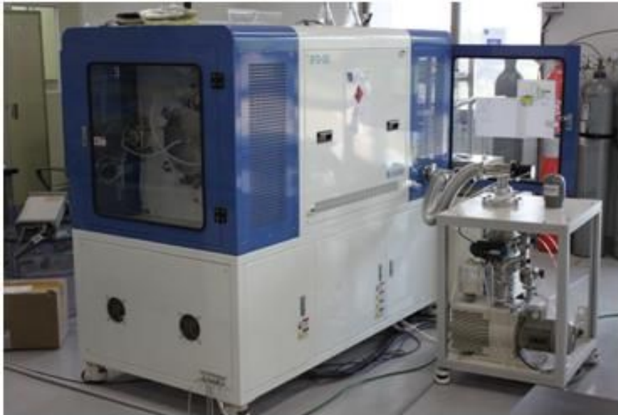
Fig. 4.2 Photograph of high vacuum furnace for corrosion test
