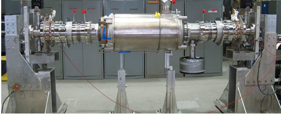
FIG. 1. (Color) The ERL cavity string.
