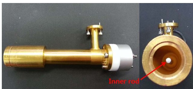
FIG. 3. Assembly of a fabricated NRMG.
