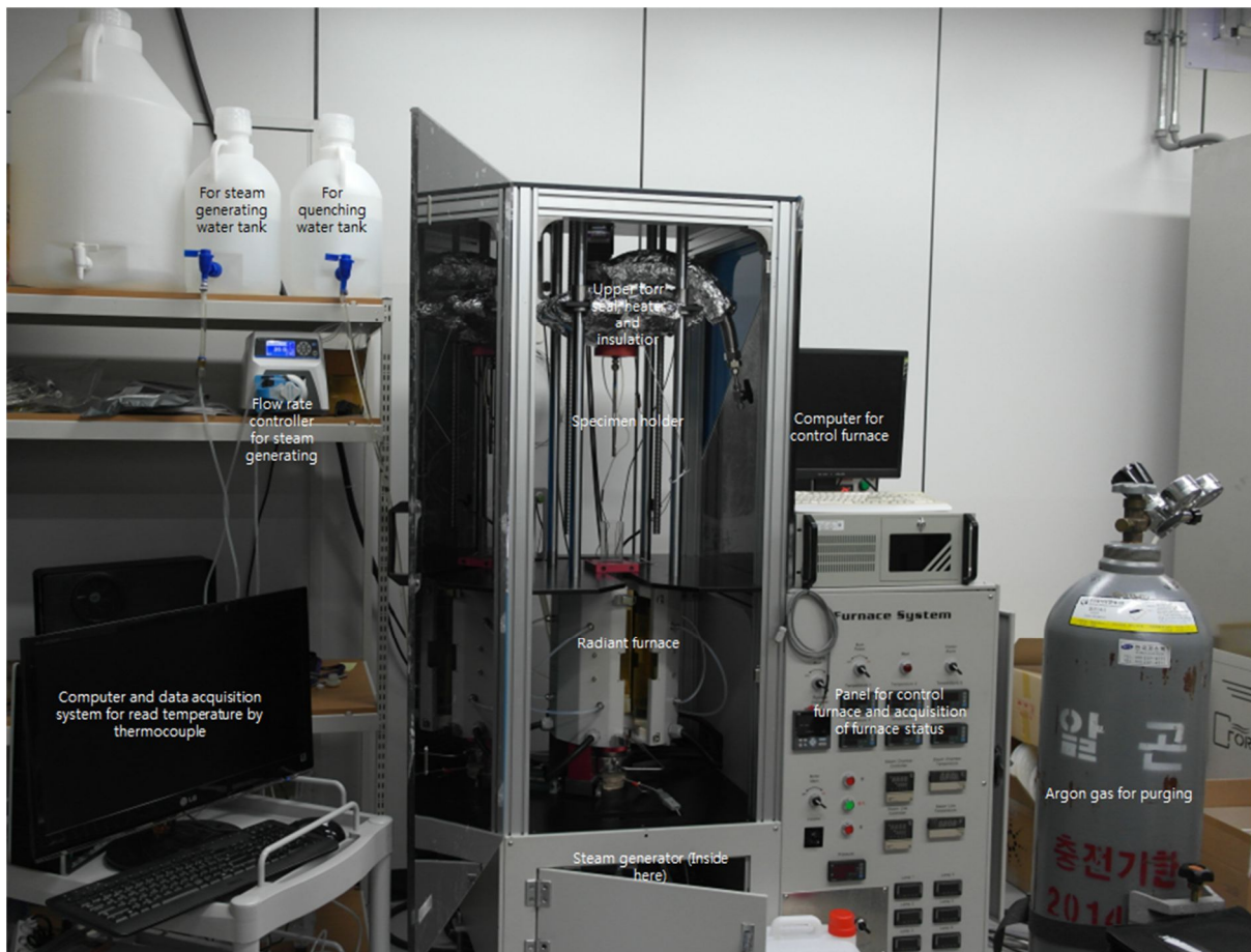
Figure III-2 Picture of the high temperature oxidation test equipment in the UNIST
