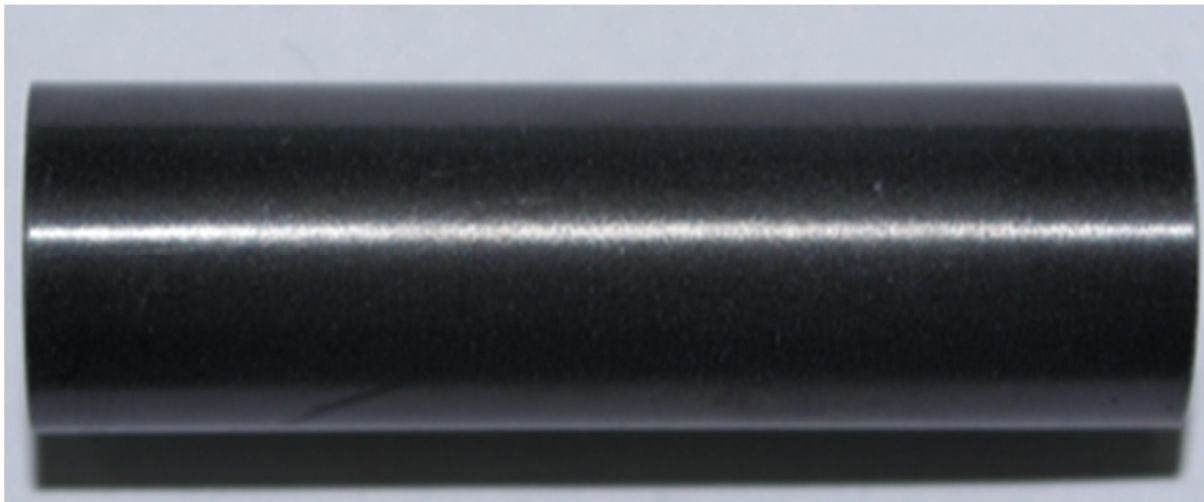
Figure III-5 Surface appearance of post-test specimen using method of steam pre-purging during 10 minutes
