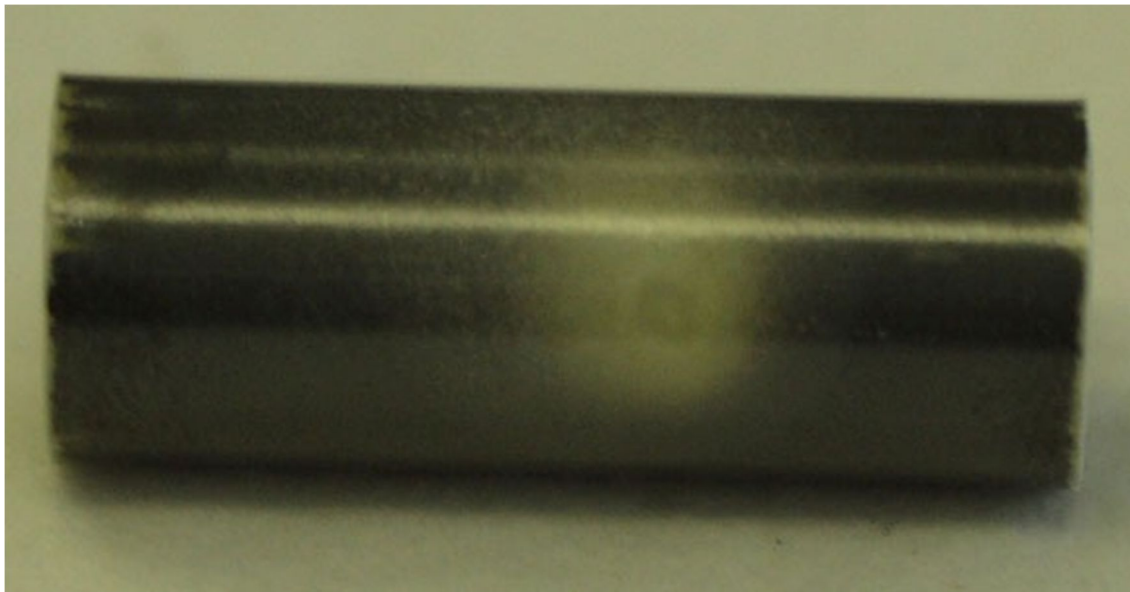
Figure II-9 White oxide on the surface can be observed after the high temperature oxidation test from conducting the test in ANL 2b
