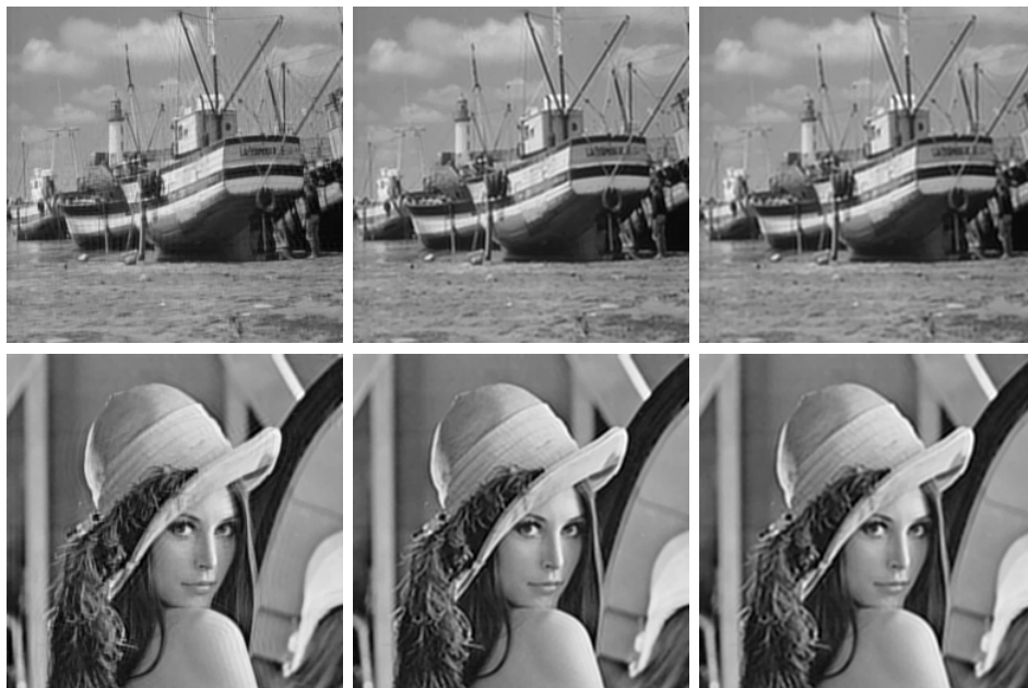
Figure 23. Comparison between the three blur types, II, V, and VI after 300 iterations. Left (type II): PSNR = 32.49 (boat) and 31.98 (woman). Middle (type V): PSNR = 31.54 (boat) and 32.60 (woman). Right (type VI): PSNR = 29.85 (boat) and 31.05 (woman).
