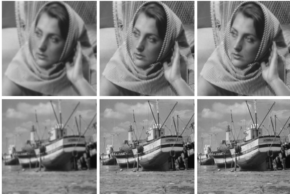
Figure 22. 7 \times 7 Gaussian blur of type V. Left: Output, PSNR = 24.75 (woman) and 26.35 (boat). Middle: Output, PSNR = 27.68 (woman) and 30.29 (boat) after 50 iterations. Right: Output, PSNR = 30.96 (woman) and 31.54 (boat) after 300 iterations.
