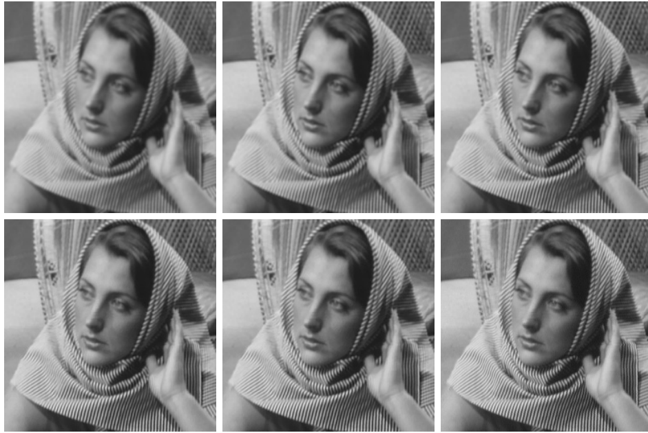
Figure 18. 3 \times 3 average kernel, blur type I. Left to right and top to bottom: Blurry image; recovered image with p = 2 , p = 1.9 , p = 1.01 , p = 1 ; original image.
