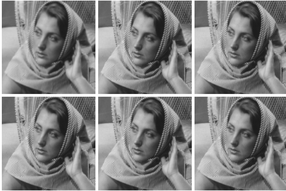
Figure 19. A closer look at the case p = 1.01 in Table 6. First row, from left to right: Blurry image, output images after 10 and 20 iterations (PSNR values: 26.49, 31.20, 32.91). Second row, from left to right: Output image after 30, 40, and 50 iterations (PSNR values: 33.76, 34.30, 34.72). Computational time for 10 iterations amounts to approximately 3.6 seconds.
