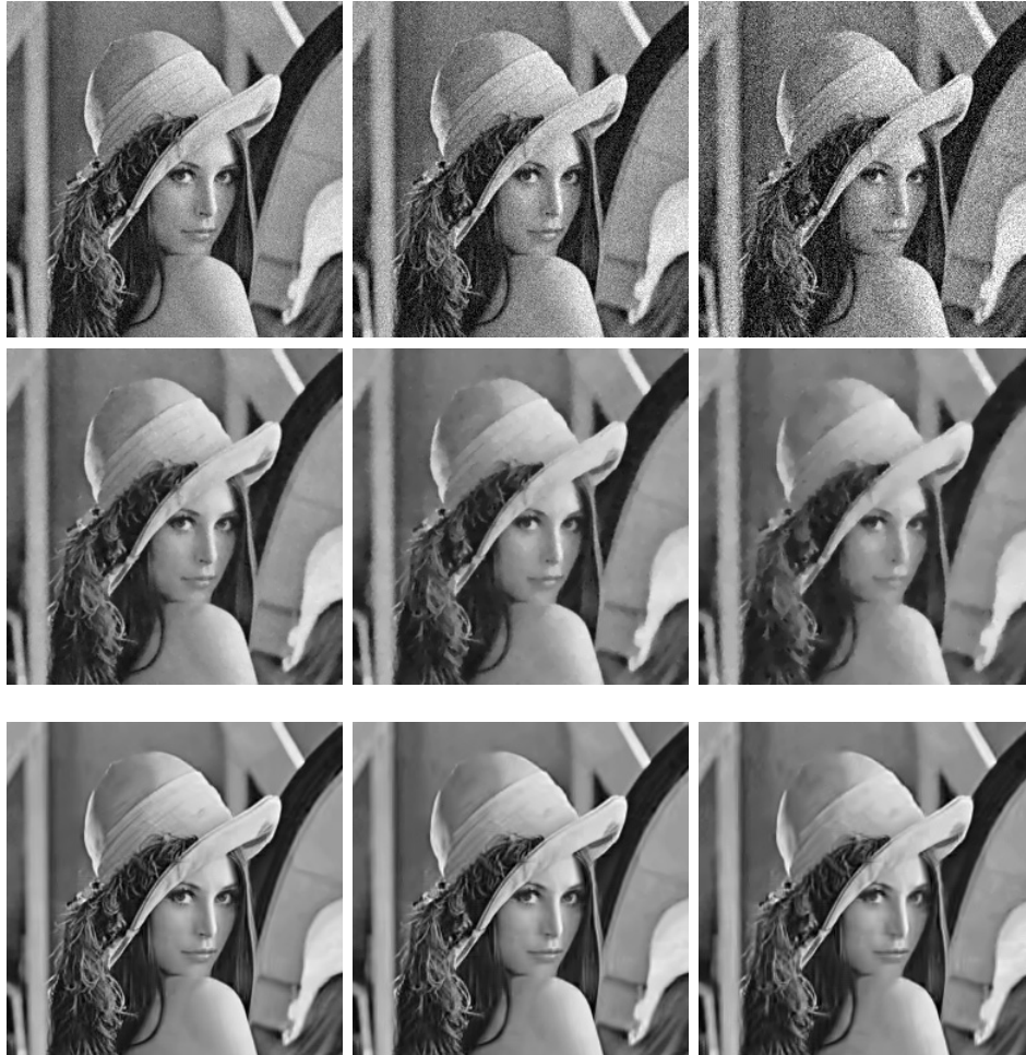
Figure 16. \delta = 0.2 , p = 1.1 , dt = 0.007 . Top row, from left to right: Noisy images with \sigma = 10, 15, 25 . Middle row: Images recovered from the noisy images right above. Bottom row: Images recovered with a state-of-the-art denoising algorithm, BM3D [4], for comparison.
