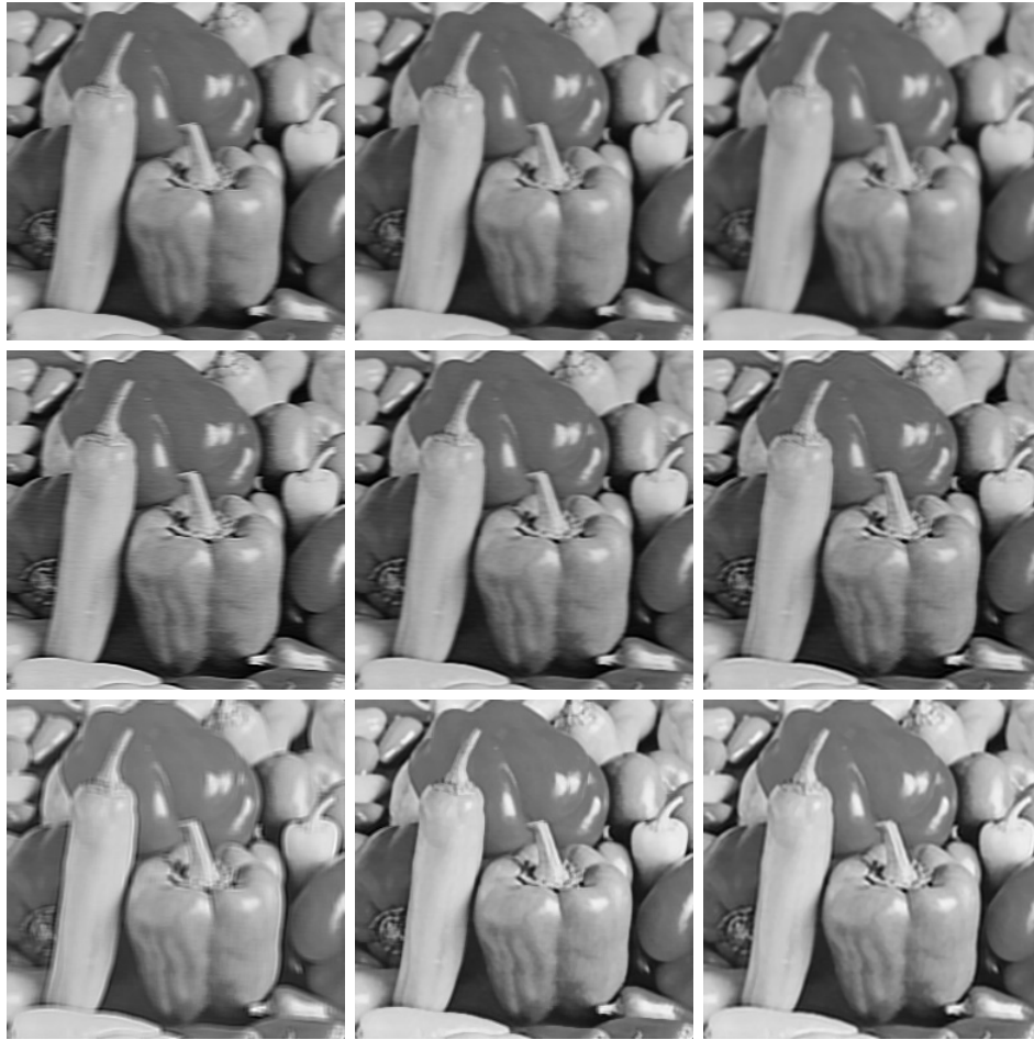
Figure 25. Recovery results. Top row: Blurry images. Middle row: Recovered images by our proposed model. Bottom row: Recovered images by the ROF model. Left column: 1 \times 5 horizontal motion blur. Middle column: 3 \times 5 blurring kernel A in Table 7. Right column: 3 \times 5 blurring kernel B in Table 7.
