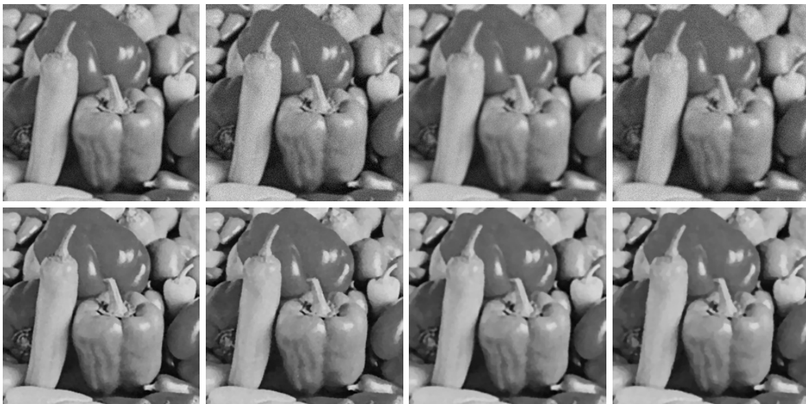
Figure 4. Top row: Noisy blurred images. Bottom row: Recovered images corresponding to the above images. Left two columns: 3 \times 3 average blur of type I and noise levels \sigma = 5, 8 , respectively. Right two columns: 7 \times 7 Gaussian blur of type V and noise levels \sigma = 5, 8 , respectively.
