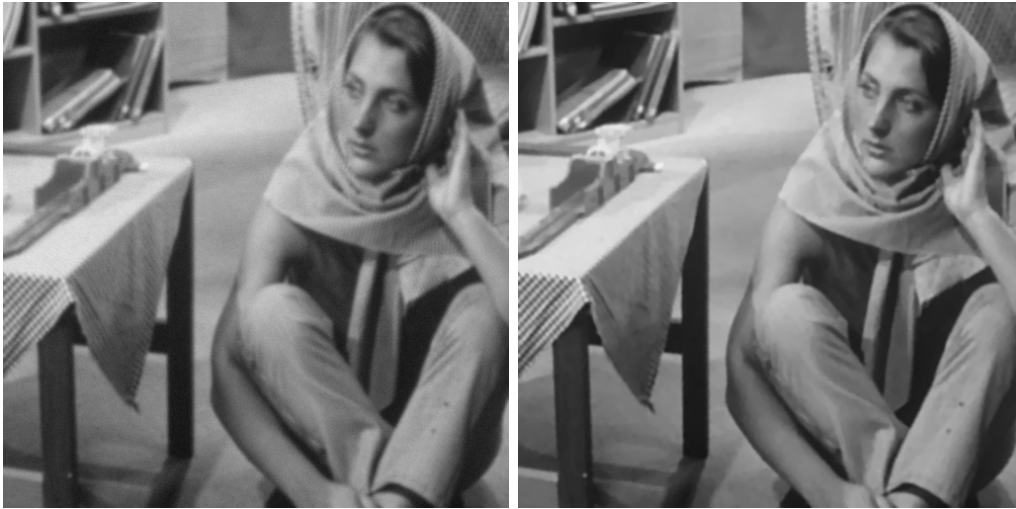
Figure 6. Recovery from a noisy blurred image of size 512 \times 512 with 15 \times 15 Gaussian blur of type VI and noise \sigma = 3 . Left: Noisy blurred image. Right: Recovered image.
