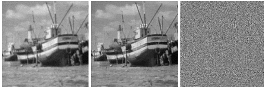
Figure 8. Left to right: Noisy blurry image ( f ) with the same blurring kernel and the same noise ( \sigma = 5 ) as in [24], restored image ( u + v ) from our proposed model, computed noise ( f - k * (u + v) ). SNR = 14.1237 , RMSE = 8.8481 .
