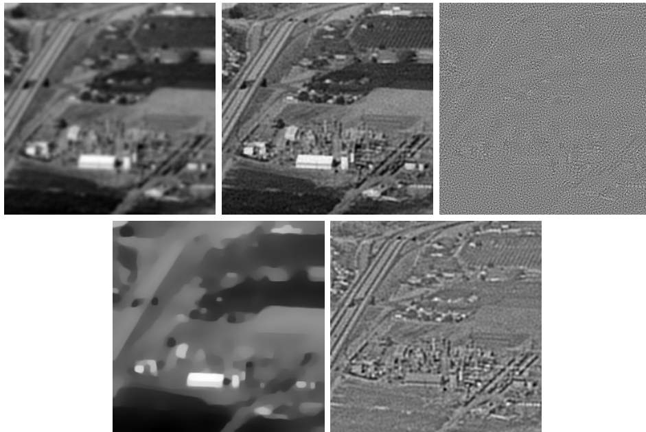
Figure 3. Top row (left to right): Noisy blurry image ( f ) with \sigma = 1.1531 , restored image ( u + v ) using the proposed method, computed noise ( f - k * (u + v) ). Bottom row (left to right): Cartoon part ( u ), texture part ( v ). SNR = 13.7362 , RMSE = 8.6380 .
