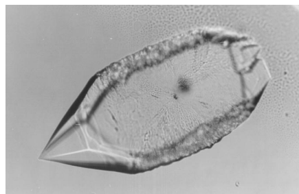
Figure 2 Hexagonal crystal of Pn-AMP1 grown in the presence of equimolar N -acetylglucosamine from citrate solution as the precipitant at 277 K. The approximate dimensions of the crystal are 0.2 × 0.2 × 0.5 mm.
