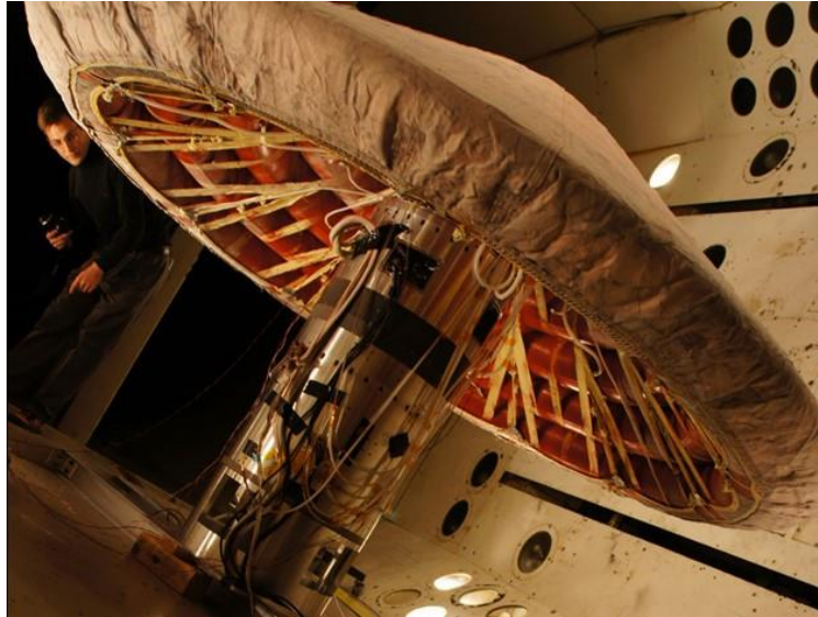
Figure 2: NASA Hypersonic Inflatable Aerodynamic Decelerator [4]
