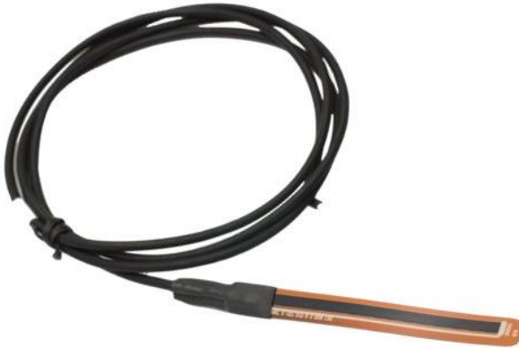
Figure 7: Flex Sensor Made With Conductive Ink [17]
