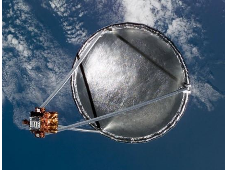
Figure 1: NASA Inflation Antenna Experiment [2]
