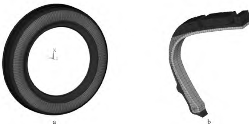
Figure 3. FE- model, a – full FE-model of tire, b – segment of tire
