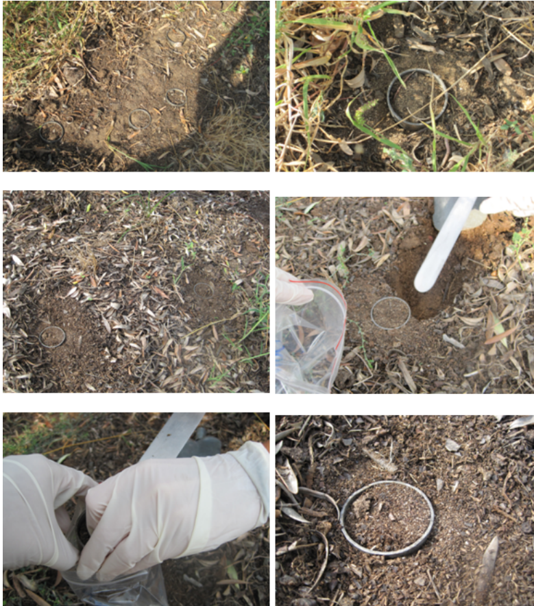
1 2 Soil sampling campaign using stainless steel cylinders
