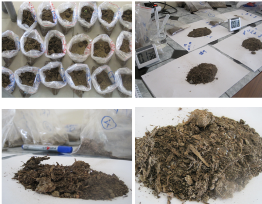
3 4 Soil water repellency measurements in the laboratory. Composted animal manure and olive 5 tree residuals are evident inside the soil matrix.
