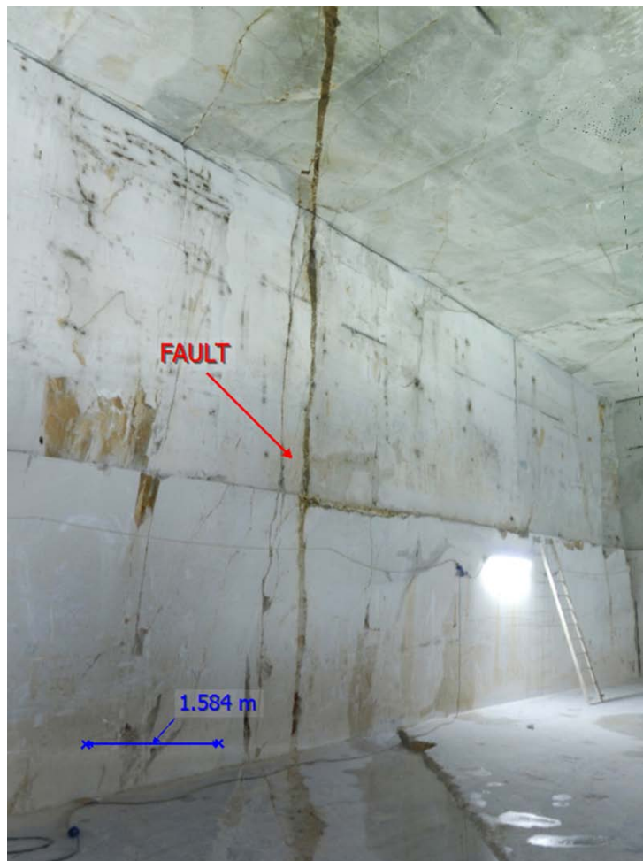
Fig. 7 Example of fault trace, the attitude of which was used to assess the reliability of single measurements by photointerpretation in VR; perspective view, the scale bar is only indicative
