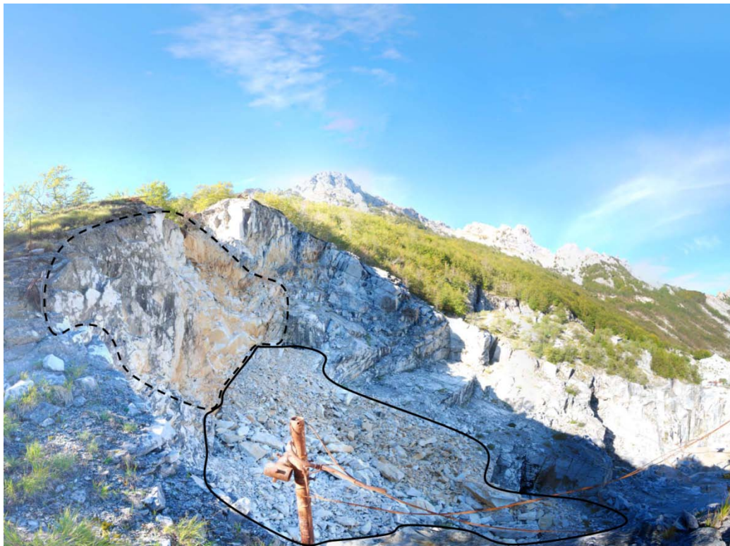
Fig. 11 Panoramic view of the rock fall that occurred at Orto di Donna quarry in 2013. Dashed line indicates the detachment zone, continuous line indicates the depositional zone
