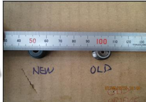
Replacement of Orifice to increase Oil flow rate
